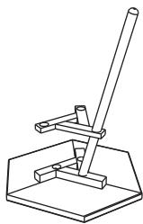
pass the star assembly through the leg with the plastic joints facing up
